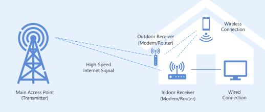
Illustration of Fixed Wireless Access connecting two fixed locations
